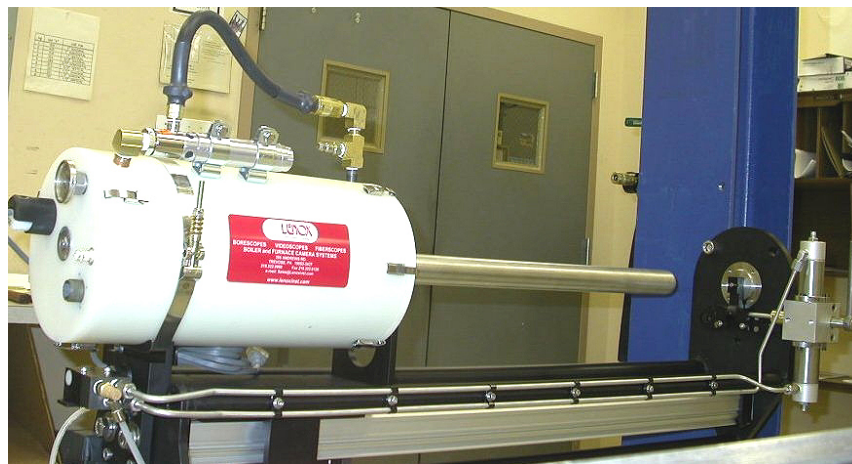
The FireSight Camera mounted on an Automatic Retract System is retracted and the Baffle is closed.
