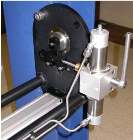
Automatic Baffle Assembly in closed position. Handle at right is for manual operation.
