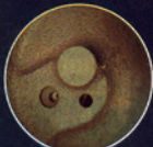
Diesel injector nozzle as seen through Lenox flexible borescope.
