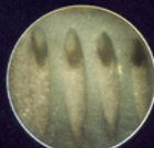
Coolant holes on turbine blade as seen through Lenox flexible borescope.
